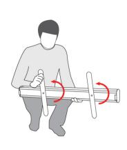
2. Assemble the three fold-pole (supporting pole) into one unit. 3. Insert the pole into the pole adapter (the hole) at the center of the aluminum base case. Large size banner stand will have 2 poles to insert.
